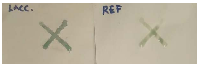
Picture 21. 10 seconds after application of substrate solution on enzyme coated surface
