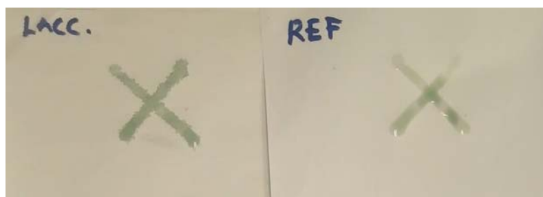
Picture 20. 5 seconds after application of substrate solution on enzyme coated surface
