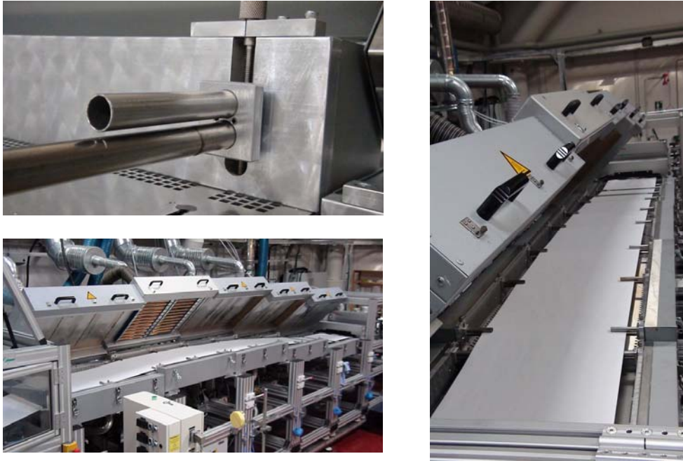
Pictures 4-6. Drying section bowed with modifications showing the solution to prevent edge curling during drying.
